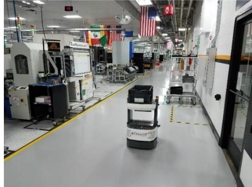
**Figure 5. Automated Material Delivery in an Automotive Electronics Manufacturing Plant**
