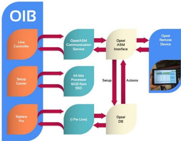
**Figure 3. ASM/Siplace Mobile Machine Control**
